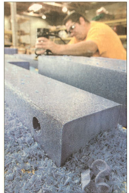
Progressive Design Playgrounds employee Charles Hayes used a router to round off the sharp edges of a recycled plastic lumber board. The board will be used in playground decking. The shavings are recycled and collected.
